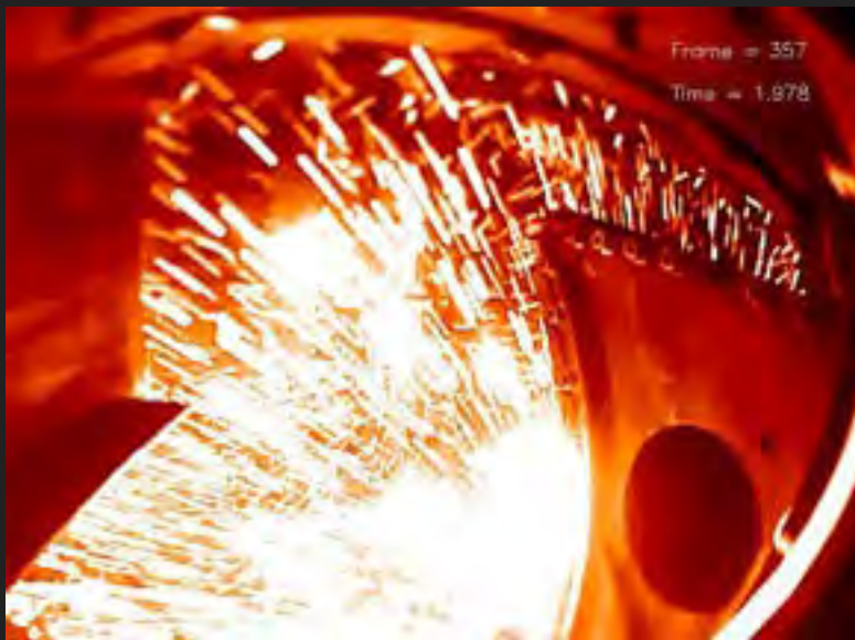
Visible camera view of RE beam hitting Alcator C-Mod first wall. Courtesy R.A. Tinguely
