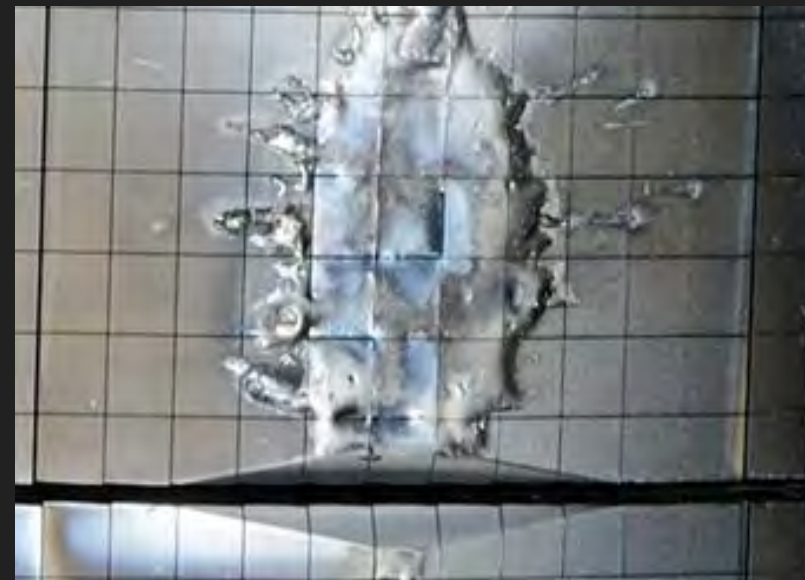
JET runaway electrons damage. https://www.iter.org/newsline/-/2234
